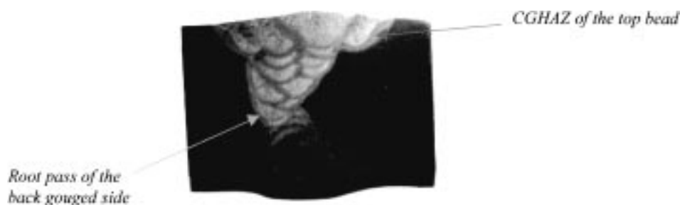
Fig. 3 Locations of microhardness indentations
