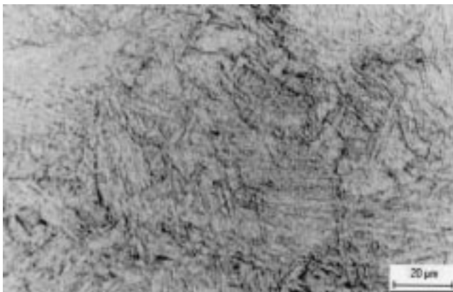
Fig. 23 OM CGHAZ microstructure of the root pass of the back gouged side (as welded)
